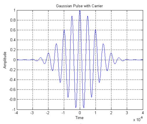
For a much higher frequency  $\omega_o = 2\pi f_o = \pi 10^7$ , the envelope is more evident
